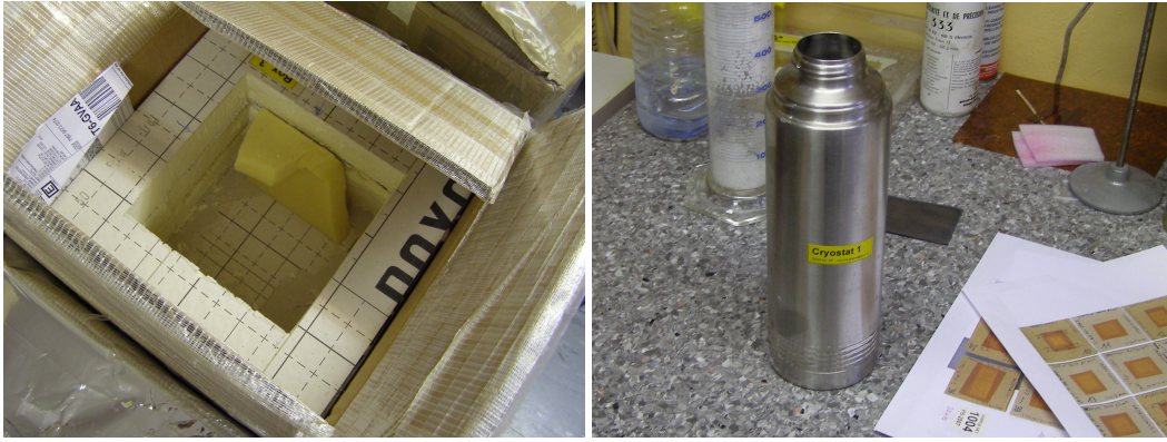
Figure 6.4: The left picture shows the transport box used for the cold transport of the irradiated samples back from CERN (provided by the irradiation facility) and the right image depicts the corresponding cryostat.
