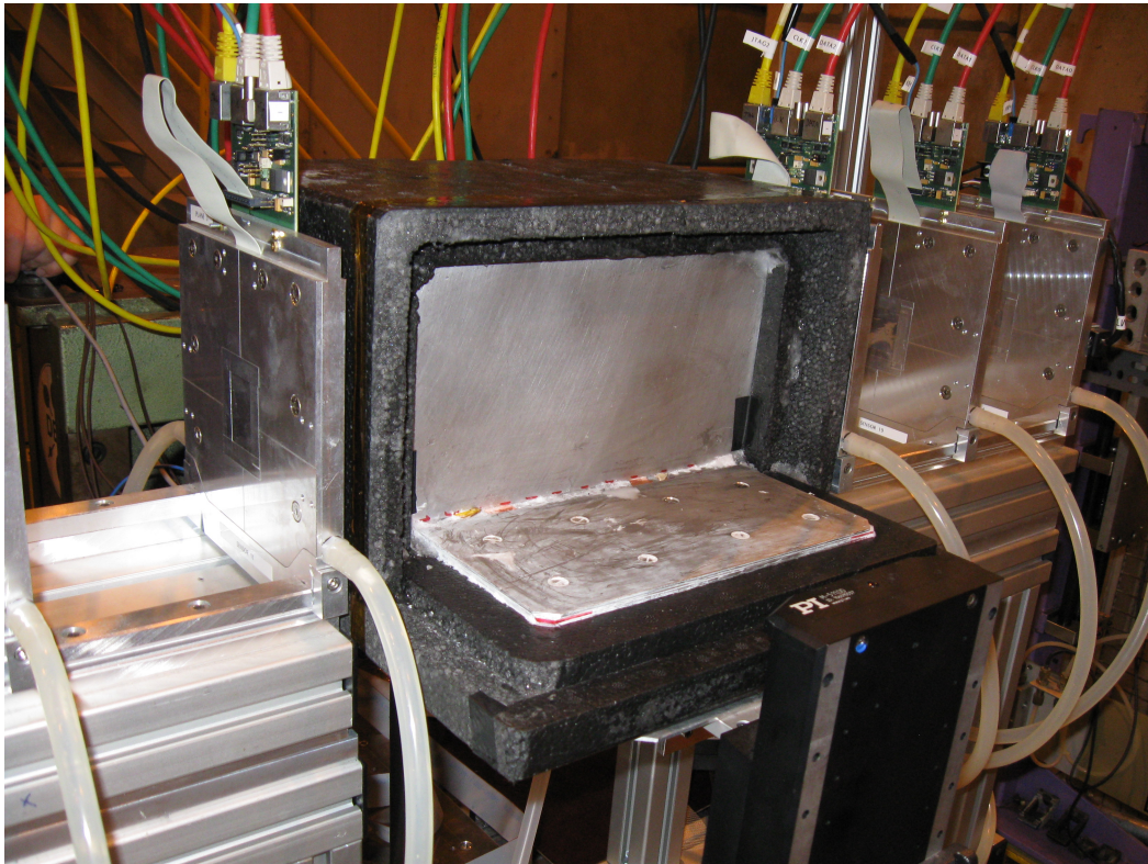
Figure 8.16: DOBOX where only the DUT compartment is closed allowing a look into the opened dry ice compartment.
