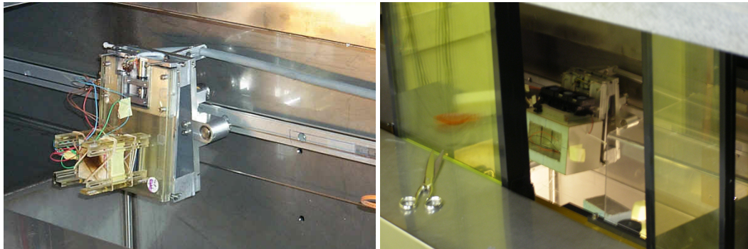
Figure 6.2: The left picture shows the shuttle (picture taken from [CER]) at PS Irrad-1 which brings the samples remotely into the beam and back, the four brackets hold the sample cardboard cards. In the right picture the shuttle is shown with the cold box installed, which enables irradiations at 0\text{ }^{\circ}\text{C} and below. One part of the samples was irradiated cold, the rest at room temperature ( 28\text{ }^{\circ}\text{C} ), as the cold box broke down due to irradiation damage of the peltier elements.
