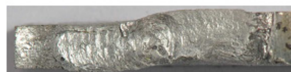
Beginning of good welding (thin weld)
