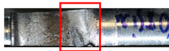
Beginning of good welding (thin weld)
