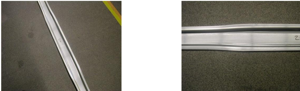
Figure 3: General view of roll formed profile (right) and close-up of the transition from narrow section to broad section.
