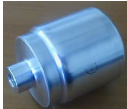
Figure 30: Al7075-T6 high pressure capsule
