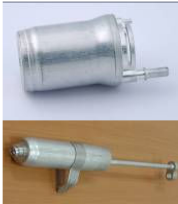
Figure 29: Al fuel filter and A/C receiver dryer
