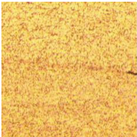
Figure 13: Ni200 etched x100
