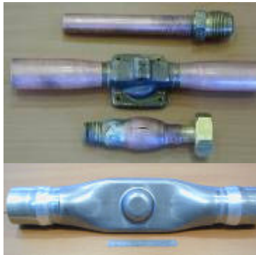
Figure 28: Cu/brass welds and Al/steel welds
