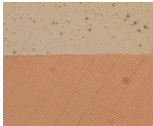
Figure 14: Al/Cu unetched x500
