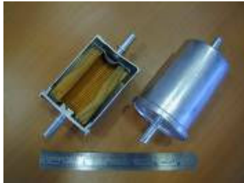
Figure 25: Al fuel filter
