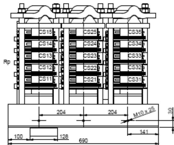
Figure 13: Design drawing of 260kA 15kVdc thyristor module
