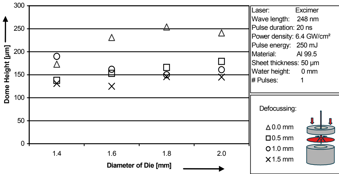
Figure 5: Dome height of laser stretch-formed parts depending on the defocussing (no water film)
