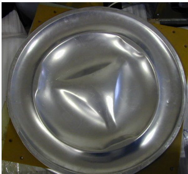
Figure 10: Formed Stainless Steel
