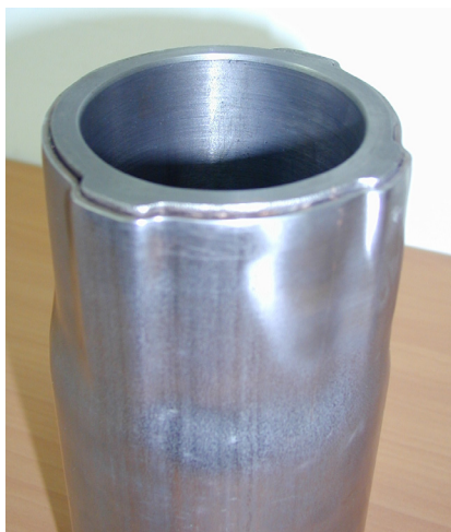
Figure 4: Tubular Forming 3 mm steel
