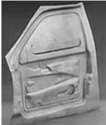
Figure 3: Inner door made from AM50 die cast (the newest VW Polo) [9]
