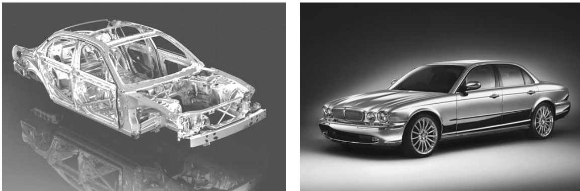
Figure 2: Self-supporting aluminum car body in Jaguar XJ [3]
