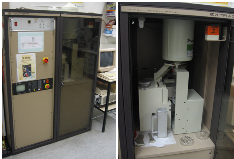
Figure 4.1.: Photos of the X-ray spectrometer EXTRA II ( Seifert, Ahrensburg, Germany; now Atomika Instruments GmbH / CAMECA GmbH, Oberschleißheim, Germany ) utilized for TXRF measurements in this work. The left picture shows the entire instrument with tube and generator section (left), measurement section with radiation protection door (center) and control computer (right). The right picture displays a more detailed view of the measurement section. The selectable Mo and W X-ray tubes are located in the boxes on the left and behind, respectively. Samples can be introduced using a sample changer box (in front). Fluorescence radiation is measured by a nitrogen cooled Si(Li) detector (above).
