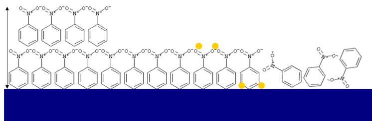
Figure 3.15.: Different possible orientations of nitrobenzene (NB) molecules and gold atoms on the substrate: The nitrobenzene molecules can form a monolayer, bilayer or multilayer. They can be ordered or disordered (with different density), and gold can stay on top of the NB layer or diffuse down to the substrate.
