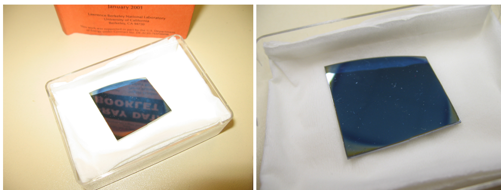
Figure 3.11.: Photos of the silicon substrate carrying a 134 nm PBMA film with silver clusters.
