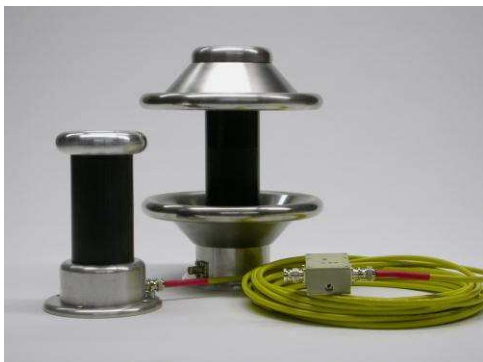
Fig. 3. Examples of high voltage dividers
