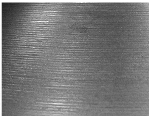
Fig. 7a. Rills caused by roller tool indentations
