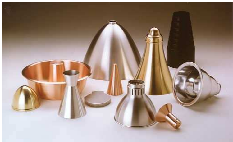
Fig. 2. Typical workpieces of shear forming, see Ott [1]
