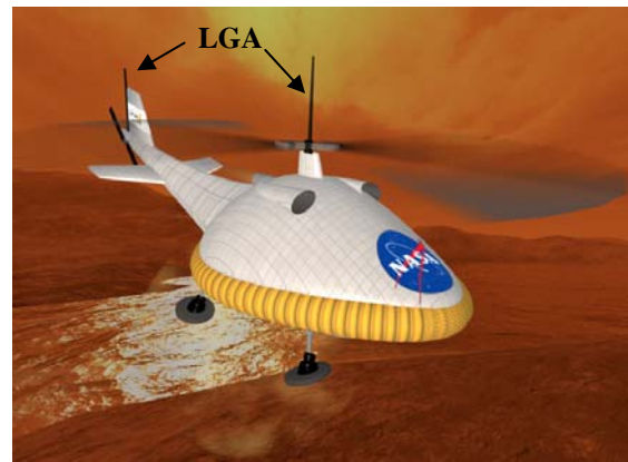
Figure 7 – Low Gain Antennas on Helicopter
