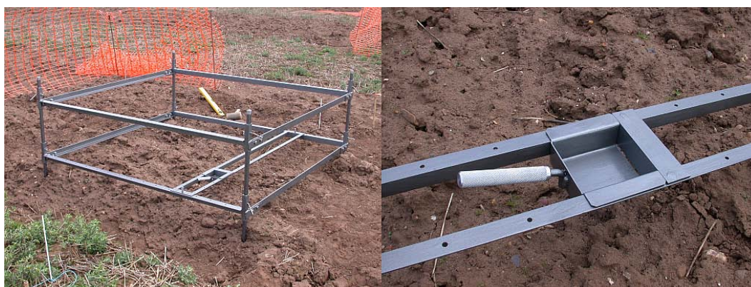
Figure 3-6 Left: excavation framework (1.5x1.5m) used to determine vertical distribution of beads after cultivations. The excavation quadrat is dropped 3 cm. each time soil in a horizontal plane has been excavated. Right: 10x10x3 cm soil blocks can be collected separately using a scoop and an insertable partitioner. Alternatively, soil blocks can be bulked for each forward position (row). The white sticks (bottom left) were inserted in line with and at known distances from the outer widths of the line of beads to mark the position before cultivation.
