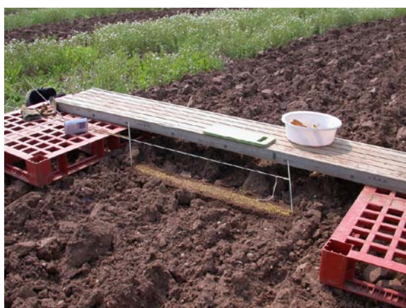
Figure 3-14 The Surface layer of beads in one of the ‘Power harrow’ plots in previously ploughed soil.
