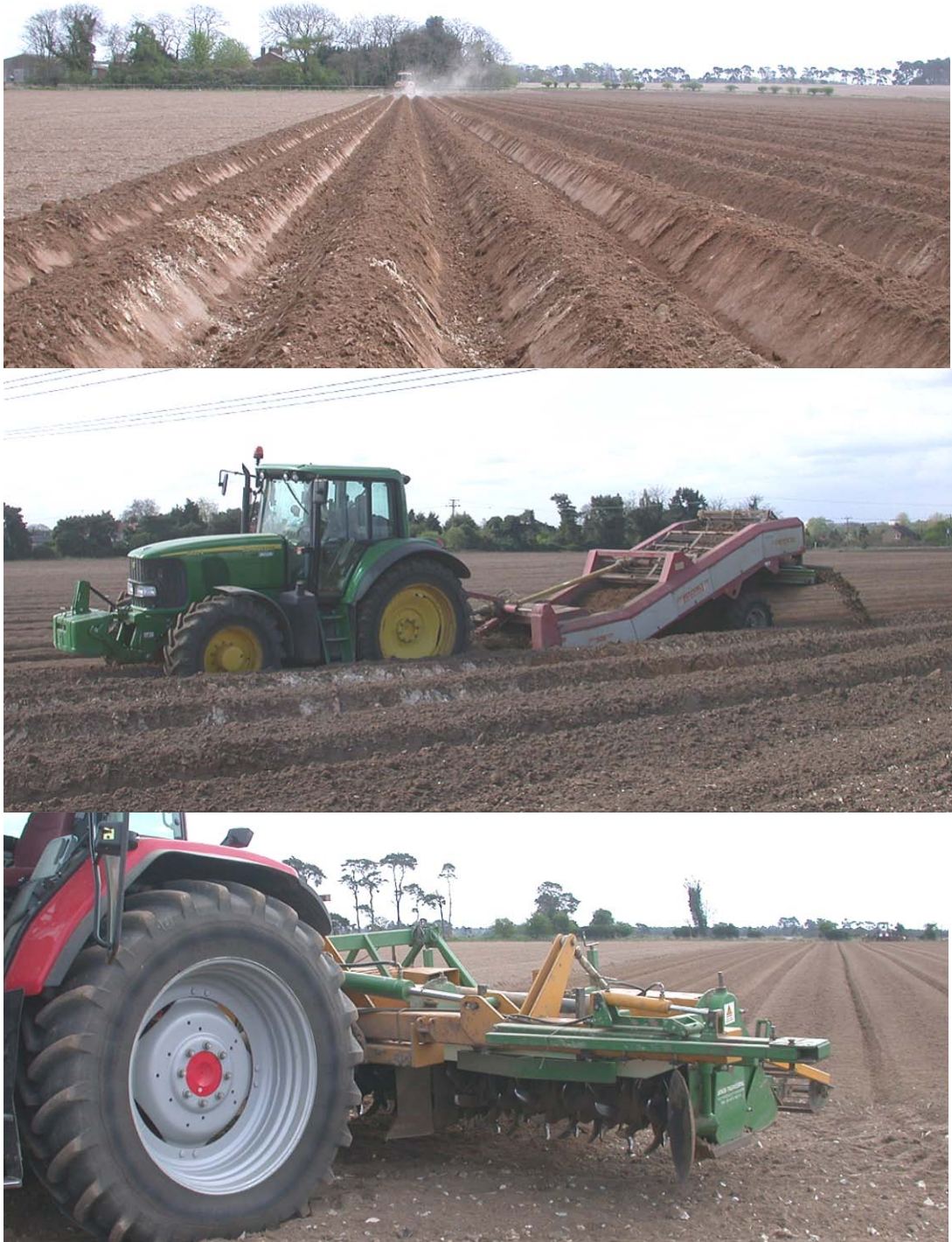
Figure 3-33 Seedbed preparation of a carrot field. Top: Ridging with a bedformer / ridger. Middle: Destoning the ridges with a stone-and-clod separator (Reekie Reliance 500); soil is taken up by a series of rotating devices that sieve the soil and deposit stones and clods in the tramlines. Bottom: Rototilled beds with Jones Engineering Triple Bedformer, now ready for carrot drilling. Images taken at Elveden Estate (Norfolk, UK) and with courtesy of Andrew Francis.
