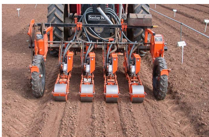
Figure 4-28 Carrot seed drilling using a Stanhay Singulaire 785. Seeds are drilled as triple rows in the compressed strips. Image courtesy of Paul Neve.
