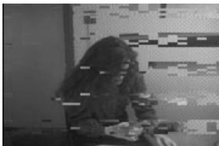
**Abb. 8.3: Multiple Dropout**
