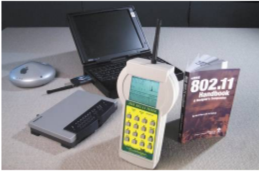
Figure 67: Berkeley-Varitronics Locust system to the left and the chosen Linksys access point to the right.
