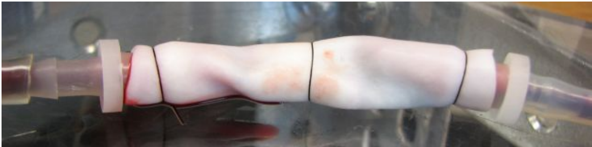
Figure 52: Test section with a patent valve, though the reservoir of blood was exhausted and the pulsatile pump was still trying to draw blood.
