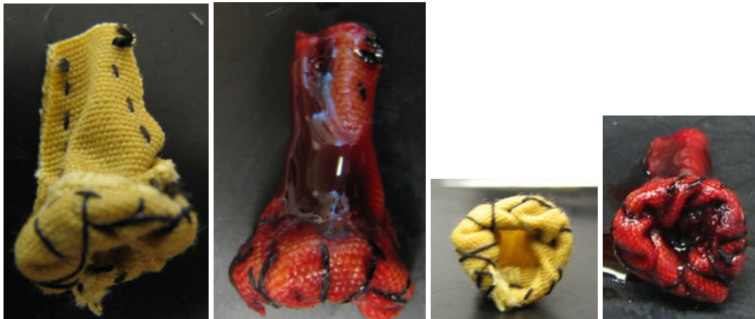
Figure 39: Longitudinal View of Dacron Sleeve (A) prior to blood flow exposure, and (B) after blood flow exposure. Cross-sectional View of Dacron Sleeve (A) prior to blood flow exposure, and (B) after blood flow exposure
