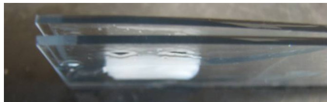
Figure 63: Flat compression of vein valve
