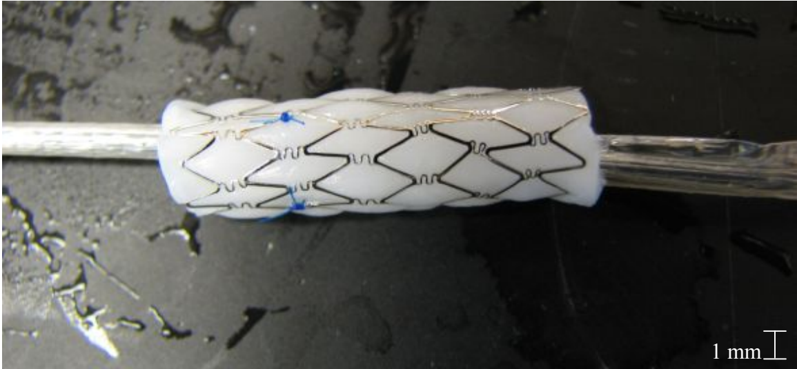
Figure 65: Radially Compressed Valve and Stent on a balloon catheter
