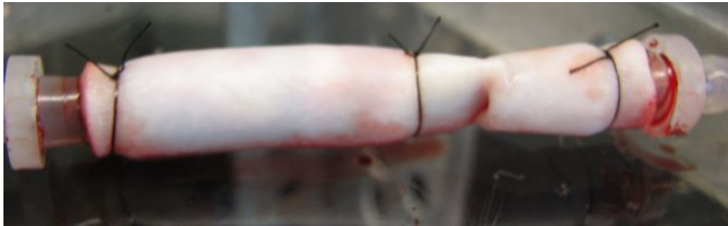
Figure 53: Test section containing a Dacron lined valve, the downstream section is collapsed due to cessation of flow.
