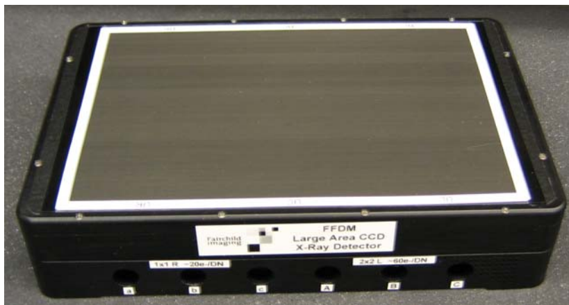
Figure 3.4. Large area 16 x 24 cm prototype imager (manufactured by Fairchild Imaging Inc., Milpitas, CA).
