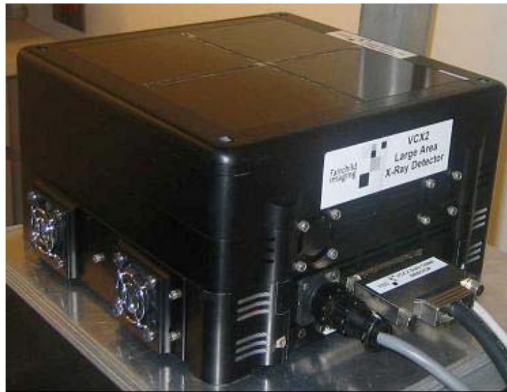
Figure 3.5. Large area 16 \times 16\ \text{cm} prototype imager for contrast enhanced mammography (manufactured by Fairchild Imaging Inc., Milpitas, CA).
