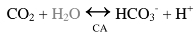
Figure 1: The conversion of CO 2 to H + and HCO 3 - is catalysed by carbonic anhydrase (CA).
