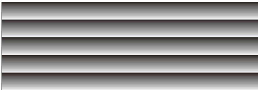
Figure 5-20: Bitmap pattern for FIB milling of blazed angle grating.
