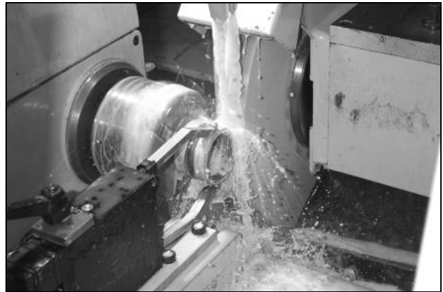
Picture of the external cylindrical grinding process and in-process gage setup in the PMRC lab at Georgia Tech.
