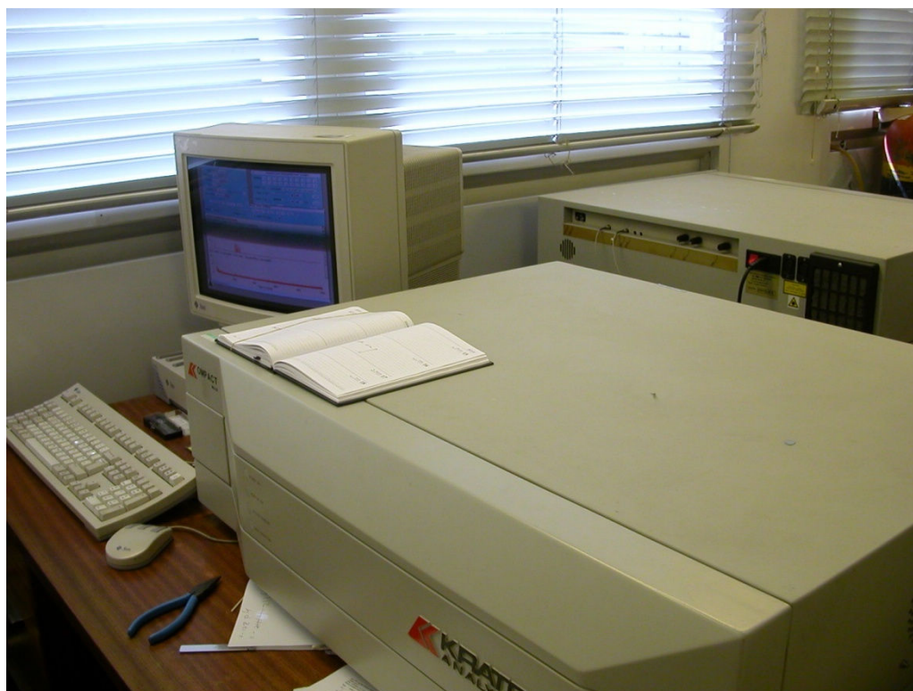
Figure 1.12: Photo of the Kratos Kompact MALDI IV
