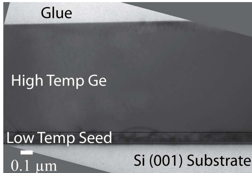
Figure 4.2: A cross sectional TEM micrograph of the control 1 \mu\text{m} Ge underlayer. Note that the low temperature seed contains a high density of dislocations.
