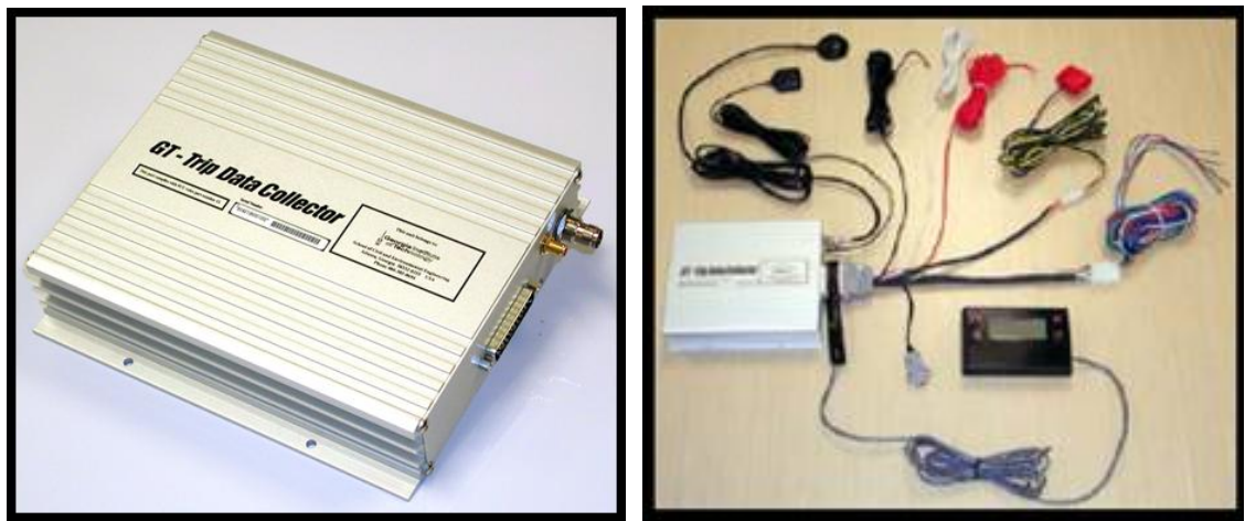
Figure 7: GT Trip Data Collector and Wiring Harnesses and Antennas
