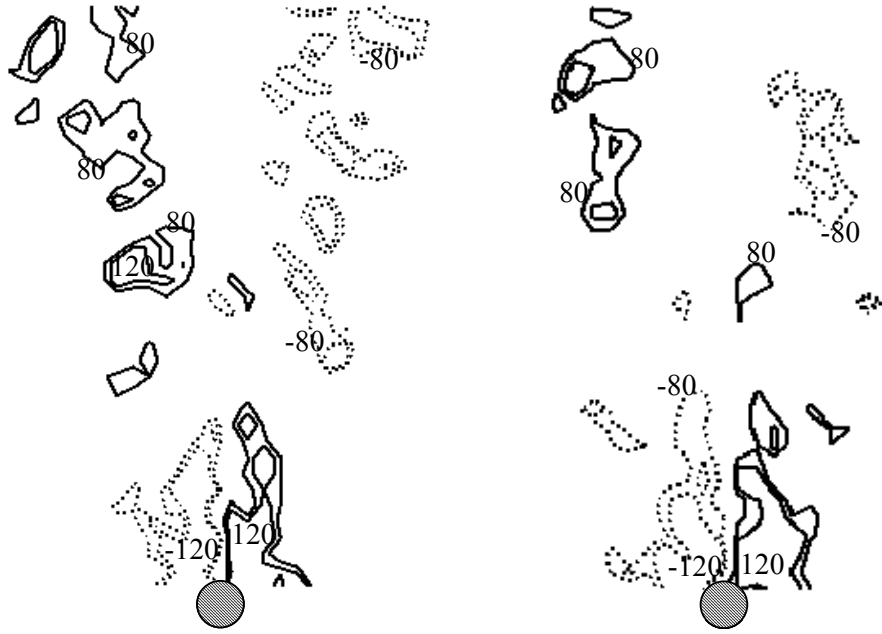
Figure 71: Instantaneous vorticity contours at 2 different instances at \phi=0.72 .
