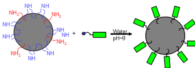
Figure 72: Grafting of the Alexa Fluor® 488 fluorescent probe on the surface of CPMs
