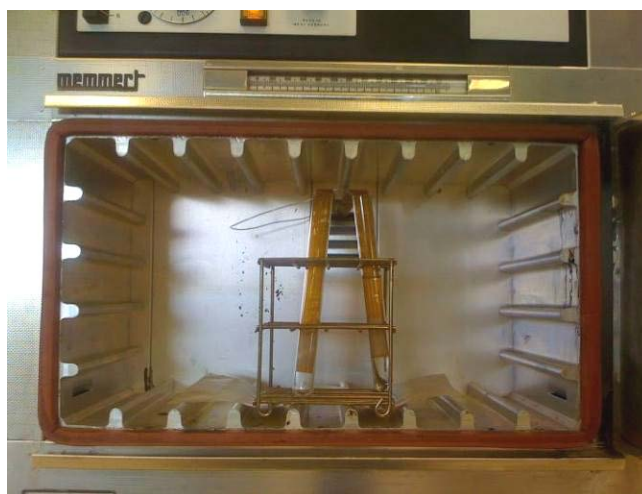
Figure 122: Image of microdielectrometry experiment - Monitoring of the CPM formation inside an oven at 100°C.
