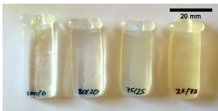
Figure II.22: PMMA (left) and PMMA/MAM samples (80/20, 75/25 and 25/75) after an annealing process at 135° C during 4 h.
