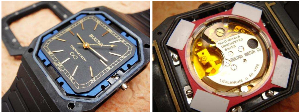
Figure I-22: The thermoelectric wristwatch Thermomatron developed by Bulova [Bul82]
