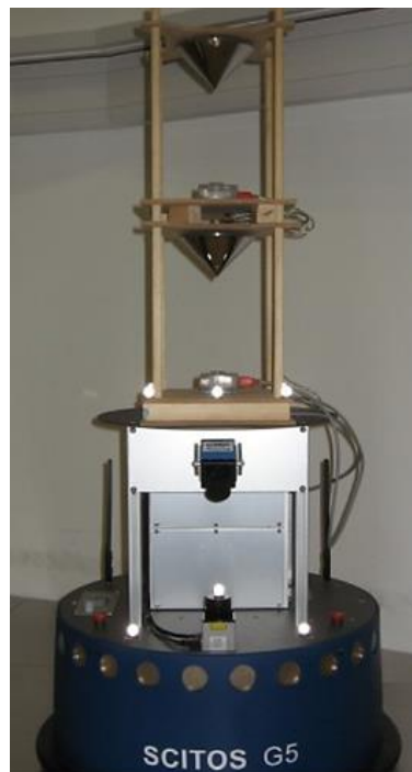
Figure 2.38: DaX, le robot mobile Scitos G5.
