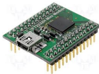
FIGURE A.16 – Le module FT2232H [84]
