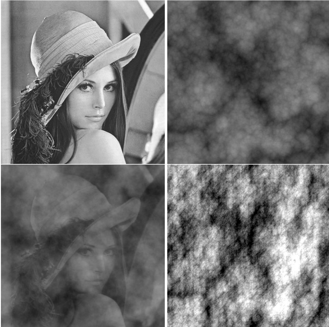
Figure 3.2: Top left: “Lena”. Top right: “clouds”. Bottom left: the Oppenheim-Lim image w as defined by (3.2), with “Lena” as u (phase) and “clouds” as v (modulus). Bottom right: the Oppenheim-Lim image w as defined by (3.2) with “clouds” as u (phase) and “Lena” as v (modulus).
