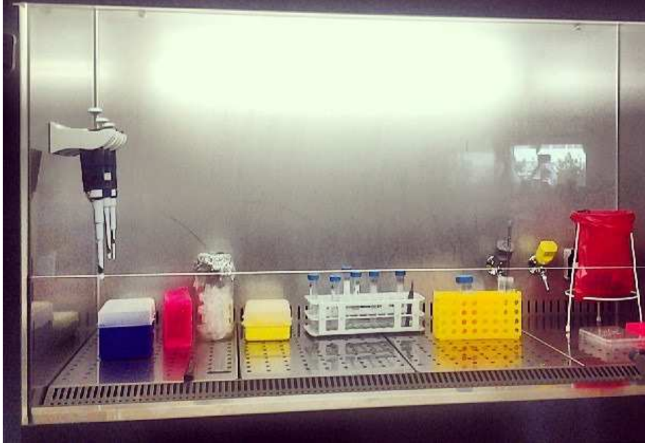
Figure II-13. Cell culture hood for the work in sterile conditions.
