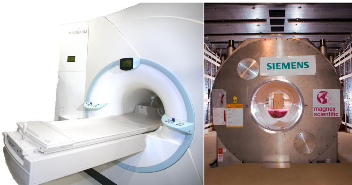
Figure 3.1: a: Siemens Magnetom 7 Tesla MRI system. b: 90-cm-diameter-bore superconducting magnet.
