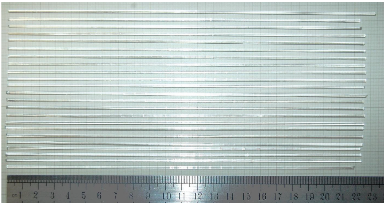
Figure IV.12. Undoped LuAG fibers with the length over 22 cm.
