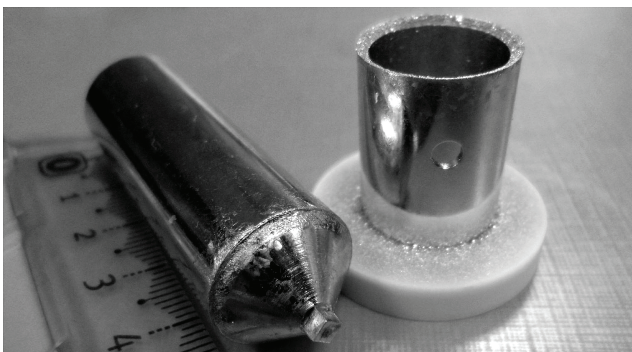
Figure II.1. Ir crucible and afterheater
