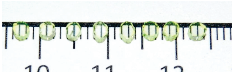
Figure IV.20. LuAG:Ce tranverse cut samples optically polished for microscopy analysis.
