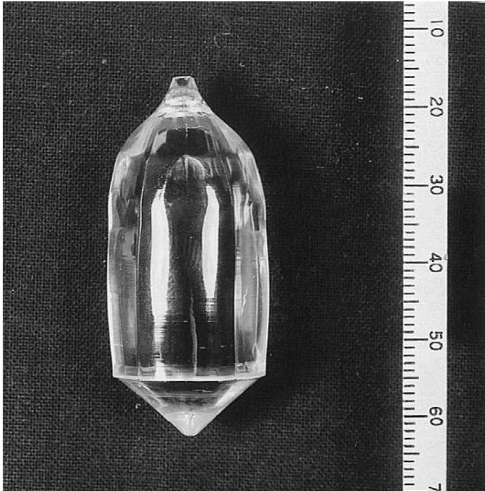
Figure I.2. Photograph of the as-grown \text{Lu}_{1.5}\text{Y}_{1.5}\text{Al}_5\text{O}_{12} single crystal [42]
