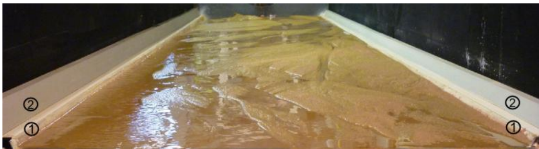
424 425 Figure 3: Topography apparatus: 1) moving rail, 2) camera, 3) video projector, 4) projected 426 fringes
