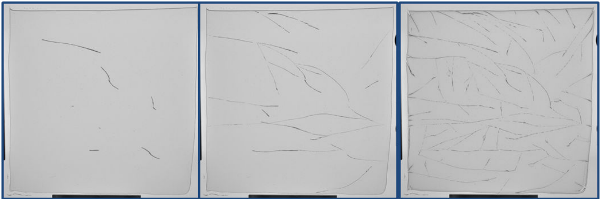
Figure .15: Time-resolved process of fracture development in the gelatine layer.
