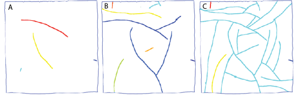
FIG. 4. The evolution of the fracture network for experiment D. Connected fractures are marked with the same color. A: New cracks nucleate. B: Fractures propagate and coalesce. C: Coalesced fractures form large connected pathway for outgoing gas.
