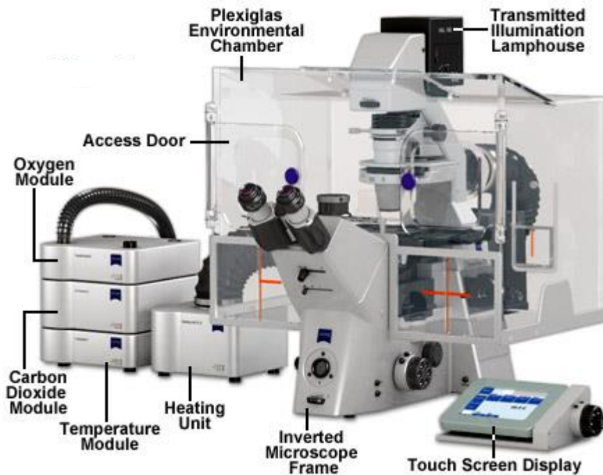
Figure 1.1: Standard lens-based time-lapse microscope. Standard lens-based time-lapse microscope setup housing an environmental chamber connected to external CO 2 , O 2 and temperature modules to provide ambient cell culture conditions.
