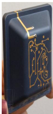
Fig. 4.63 : Three dimensional PIFA antenna on LCP Vectra E820i, (a) simulated structure and (b) fabricated photo.
