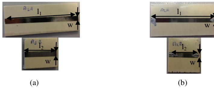
Fig. 5.35 : Microstrip transmission lines on planarized LCP E130i with different metallization thickness (a) with 0.7 \mu\text{m} , and (b) with 1.4 \mu\text{m} .
