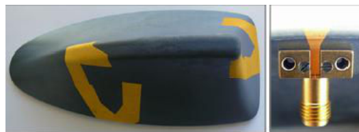
Fig. 2.30 : Realized two antennas system (LTE and automotive roof top antenna) with feeding structure on MID.
