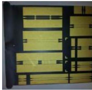
Fig. 4.3: LDS fabricated circuits on a molded LCP Vectra E820i.
