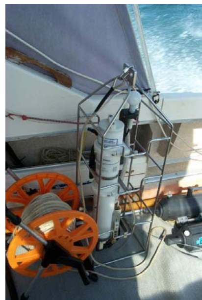
Figure II- 2 La sonde CTD SBE 19
