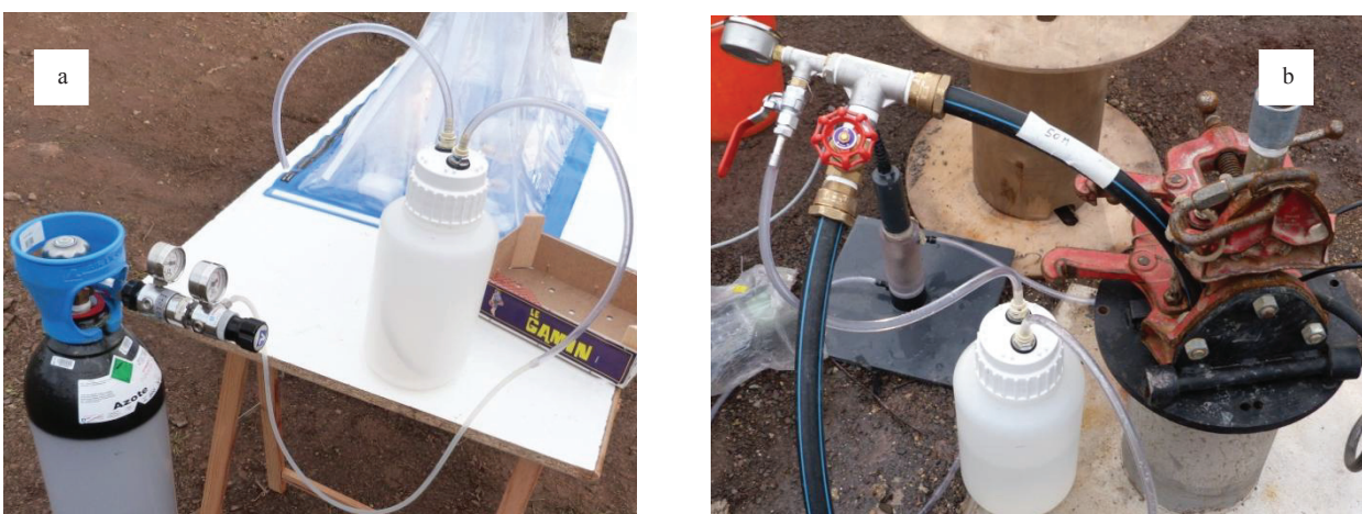
Fig. 3.2.15: (a) 4 liters bottle filled up by inert gas \text{N}_2 , (b) sampling was performed directly at the wellhead
