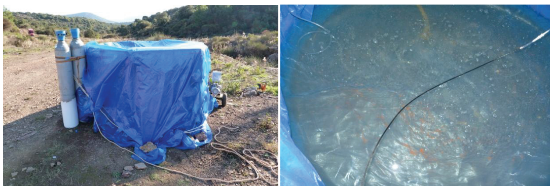
Fig. 3.2.13: water tank used for CO 2 diffusion (left picture), interior of the water tank during the CO 2 diffusion (right picture).
