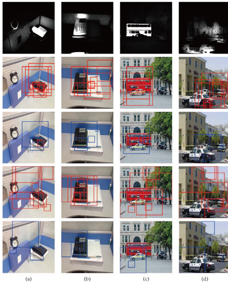
Figure 20: The salient foreground objects detection and classification results of (a) clock, (b) phone, (c) patrol car and (d) police car.
