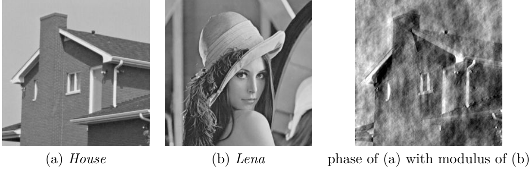
Figure 4.1: Phase and perceived geometric content. When an image is built (in Fourier domain) with the phase of an image (a) and the modulus of an image (b), the perceived geometry is that of (a). This famous experiment of Oppenheim and Lim [Oppenheim & Lim 1981] shows that the geometry of an image is mostly encoded in the phase component.
