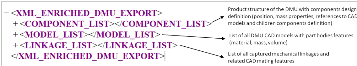
Figure 184: Structure of the DMU exported XML file
