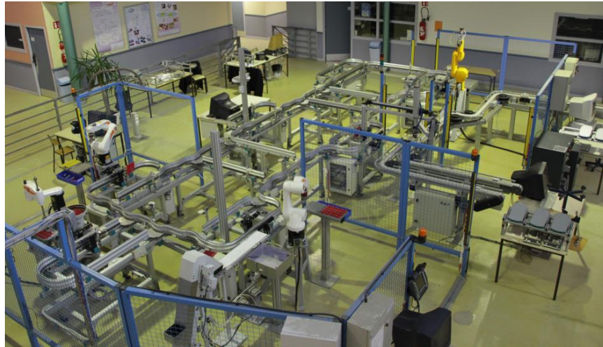
Figure V-1: The AIP-PRIMECA assembly cell
