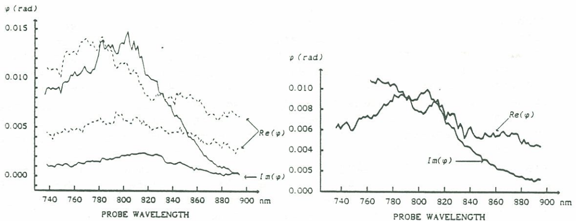
a) b) Figure 4: 100ps induced mid-gap phase shifts in 1g/l red solution: after 1.5 \text{ GW cm}^{-2} (lower curves) and 3.0 \text{ GW cm}^{-2} (upper curves) excitation at 1064nm (a-left), and after 0.25 \text{ GW cm}^{-2} excitation at 532nm (b-right).
