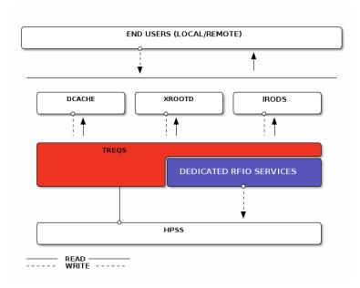
Figure 3.8: Overview of the hierarchical storage infrastructure of the IN2P3 Computing Center.
