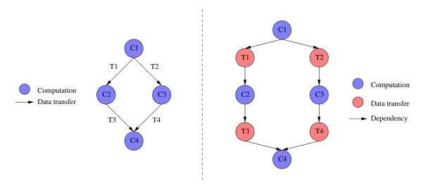
Figure 2.4: Scheduling literature and SIMGRID representations of an application structured as a DAG.
