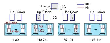
Figure 3.5: Modeling the *graphene* cluster: rectangles represent capacity constraints. Grayed rectangles represent constraints involved in a communication from node to node 40 to node 104.
