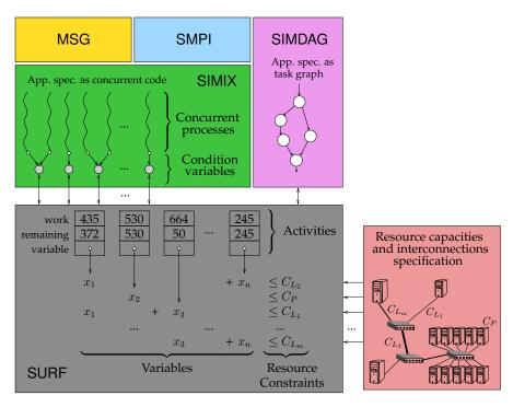
Figure 2.3: Design and internals of SIMGRID.
