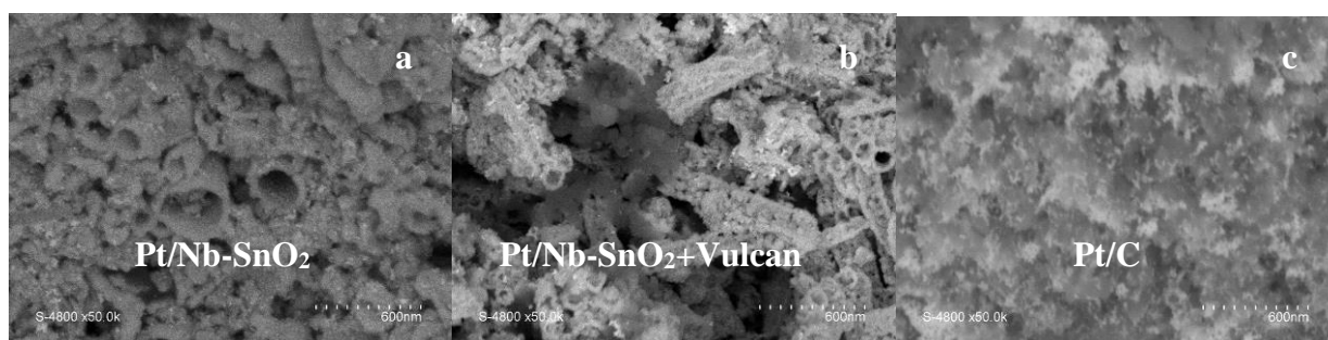
Figure 11: BSE-SEM images of 21 % Pt/Nb-SnO 2 (a), 20 % Pt/Nb-SnO 2 -Vulcan (b), and 50 % Pt/C (c) based cathode after 1200 cycles.
