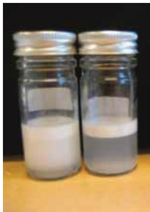
Figure 2. Emulsions stabilized using PLA- b -PEG block copolymer particles with 20% w/v of oil and 3% w/v of nanoparticles. Left: emulsion obtained using the conventional emulsification process, Right: emulsion obtained using the spontaneous emulsification process.
