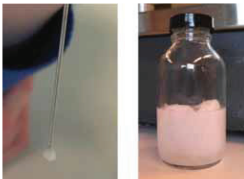
Figure 3. Emulsion (80% Miglyol 812N, 9% block copolymer): high viscosity of the organic solution (block copolymer +oil) caused clogging of the needle and leakage of the oil in the spontaneous emulsification process.
