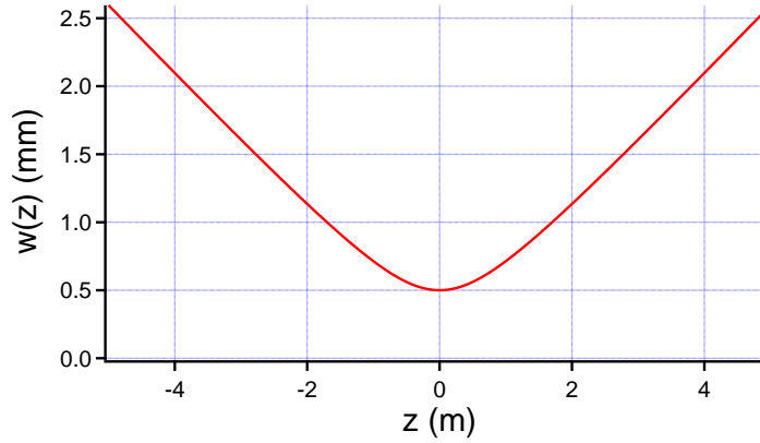
Figure 1.1: Evolution of the width w(z) of a Gaussian beam of waist w_0 = 500 \mu\text{m} at a wavelength of 800 nm.
