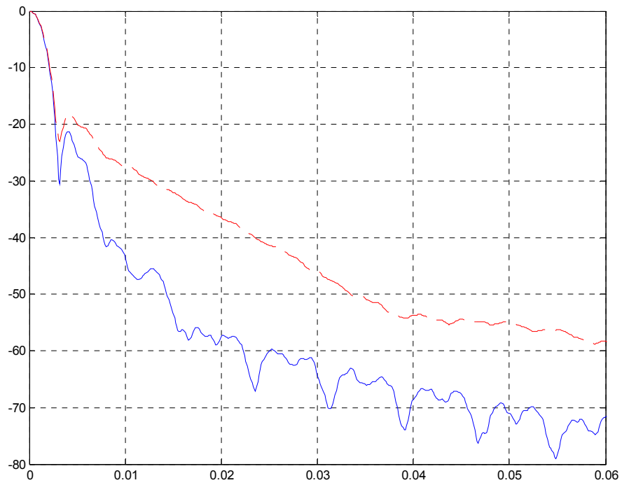
Figure 82 – ELD-AAC prototype (blue), LONG_STOP synthesis window (red)
