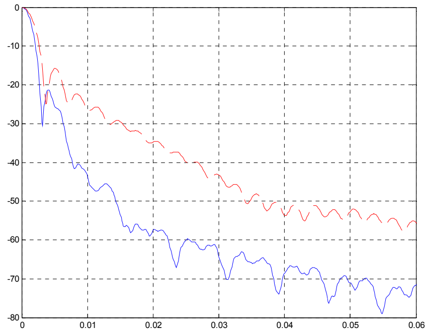
Figure 81 – ELD-AAC prototype (blue), LONG_START synthesis window (red)
