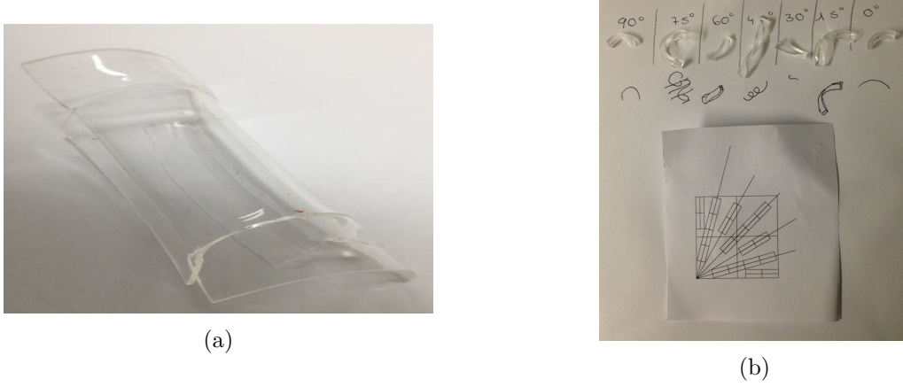
Figure 6.11 – (Left) Saddle-shaped configuration of a biaxially stretched elastomer. (Right top) Different helical configurations are obtained depending on the cutting angle of elongated strips. (Right bottom) Cutting pattern. This experiment reproduces the results of (Chen et al. 2011).
