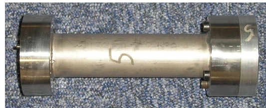
Figure 2.4 – Tube de 200 mm diam. 30mm (f+b=185mm+15mm)
